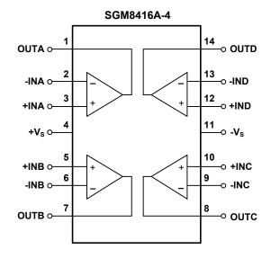
NOTE: Connect thermal die pad to -V<sub>S</sub>. Connect it to -V<sub>S</sub> plane to maximize thermal performance.
